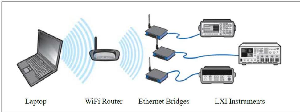
After the device has powered up and a connection to the LAN has been established, an attempt will be made to obtain an IP address as part of its boot-up process. The LXI specification requires every LXI device have a LAN status indicator. Once the connection status is good, this indicates that the LXI device has successfully booted up, obtained an IP address and can be discovered on the network.
